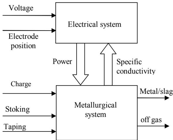
Figure (2) Complete model of the EAF system
