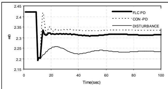
Figure (9-1) Impedance inside EAF electrode 1
