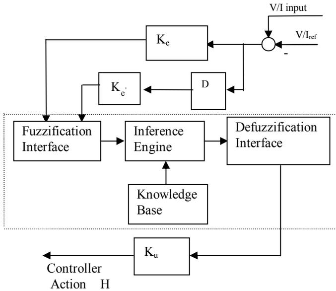
Figure (7) PD controller I/O description
