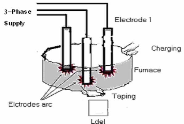
Figure (1) Schematic diagram of a submerged arc furnace
