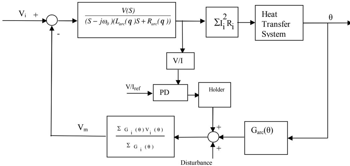
Figure (6) Closed loop system of EAF with PD controller
