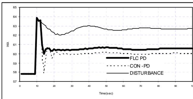
Figure (9-2) Current inside EAF electrode 1
