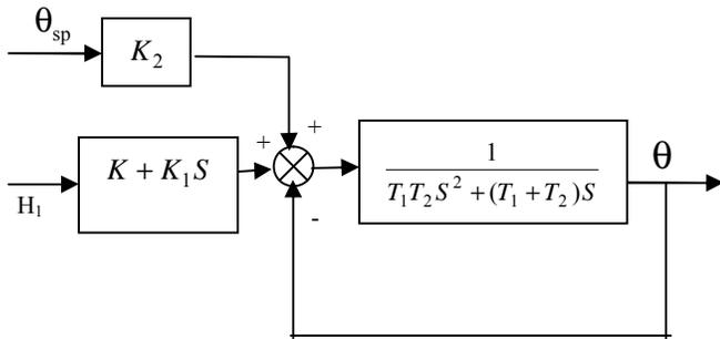
Figure (3) Heat transfer model for the electrical arc furnace
