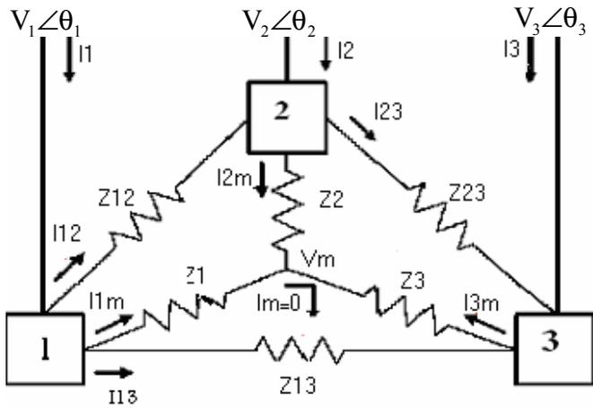
Fig (5) Electrical model of EAF
